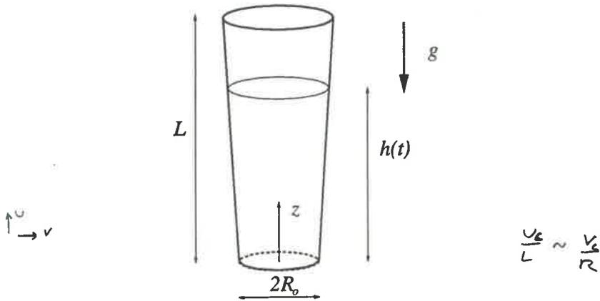
$$\rho \frac{\partial u}{\partial t} + \rho u \frac{\partial u}{\partial z} + \rho v \frac{\partial u}{\partial r} = - \frac{\partial (p + \rho g z)}{\partial z} + \mu \frac{1}{r} \frac{\partial}{\partial r} \left( r \frac{\partial u}{\partial r} \right)$$
