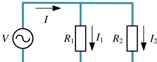
$$I_1 \cdot R_1 = I_2 \cdot R_2; \quad I = I_1 + I_2$$
