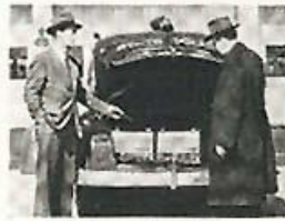
A standard mobile transmitting and receiving unit in use by Michigan State Police.
