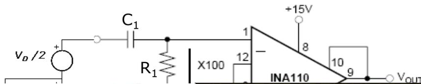
$$V_e|_{CM} = V_{CM} \left( \frac{j\omega R_2 C_2}{1 + j\omega R_2 C_2} - \frac{j\omega R_1 C_1}{1 + j\omega R_1 C_1} \right)$$
