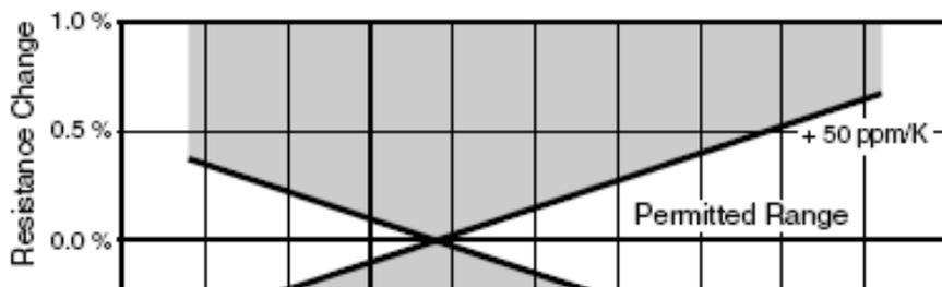
$$TCR = \frac{R_T - R_{20^\circ C}}{R_{20^\circ C} (T - 20^\circ C)} 10^6 (\text{ppm}/^\circ C)$$
