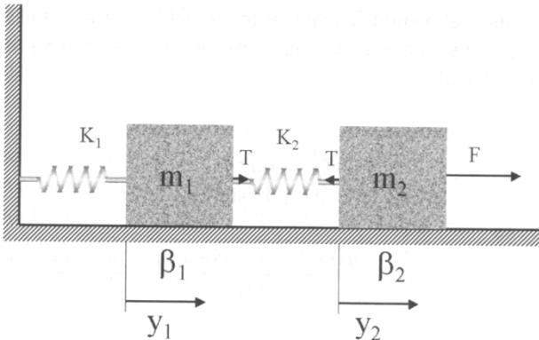
$$\begin{aligned} T &= m_1 \ddot{y}_1 + \beta_1 \dot{y}_1 + K_1 y_1 & (m_1 s^2 + \beta_1 s + K_1) y_1 &= T \\ T &= K_2 (y_2 - y_1) & s[(m_1 s + \beta_1) y_1] &= T - K_1 y_1 \\ F &= m_2 \ddot{y}_2 + \beta_2 \dot{y}_2 + T & x_1 &= (m_1 s + \beta_1) y_1 \\ & & \dot{x}_1 &= T - K_1 y_1 \end{aligned}$$
