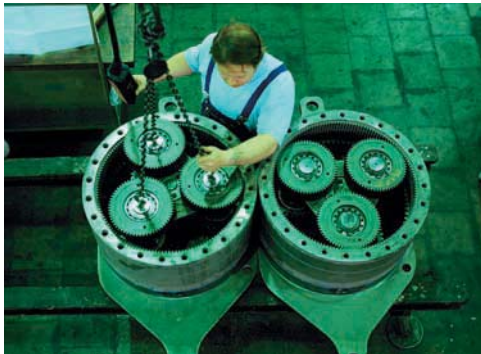
Photo 15.4 Planetary gear systems are used to high reduction ratios with minimum space and weight. The small gears undergo general plane motion.
