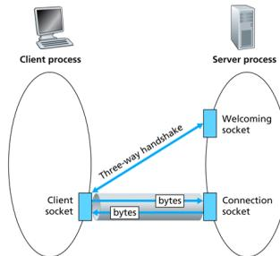
Figure 2.28 ♦ Client-socket, welcoming socket, and connection socket
