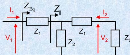
$$Z_{||} = Z_2 \parallel (Z_1 + Z_0) = \frac{Z_2(Z_1 + Z_0)}{Z_0 + Z_1 + Z_2}$$
