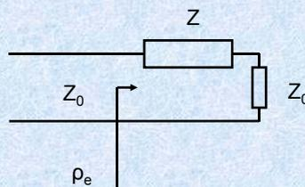
$$s_{11} = \left. \frac{b_1}{a_1} \right|_{a_2=0} = \rho_e = \frac{Z + Z_0 - Z_0}{Z + Z_0 + Z_0} = \frac{Z}{Z + 2Z_0}$$
