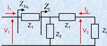
$$s_{21} = \left. \frac{V_2^-}{V_1^+} \right|_{V_1^- = 0} = \frac{V_2}{0.5(V_1 + Z_0 I_1)}$$
