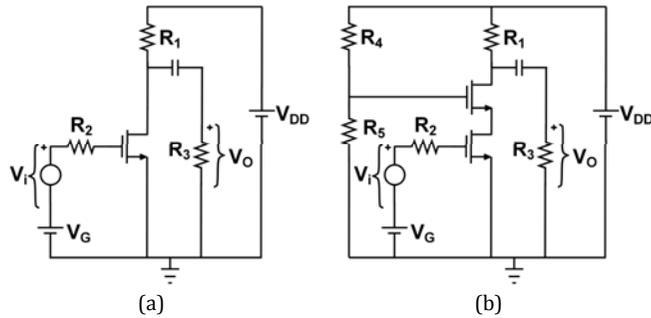
$$V_{DD} = 24V, V_G = 3V, R_1 = 5k\Omega, R_2 = 1k\Omega, R_3 = 20k\Omega, R_4 = 7k\Omega, R_5 = 5k\Omega$$
