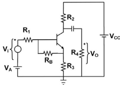
$$\beta_f = 200, V_{CC} = 12V, V_A = 10V, R_B = 2k\Omega, R_1 = 15k\Omega, R_2 = 1k\Omega, R_3 = 0.5k\Omega, R_4 = 5k\Omega$$
