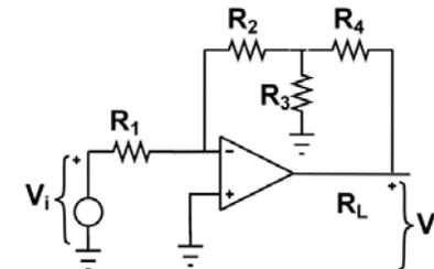
$$R_1 = 2k\Omega, R_2 = 1k\Omega, R_3 = 15k\Omega, R_4 = 6k\Omega$$
