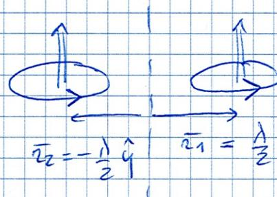
$$\begin{aligned} \bar{E}_{\text{total}} &= E_0 \sin \theta \hat{\phi} \frac{e^{-ikz}}{2} \left[ e^{+ik\bar{z}_1 \cdot \hat{z}} + e^{ik\bar{z}_1 \cdot \hat{z}} \right] \\ &\quad \left[ e^{ik\frac{\lambda}{2} \sin \theta \cos \phi} + e^{-ik\frac{\lambda}{2} \sin \theta \cos \phi} \right] \end{aligned}$$
