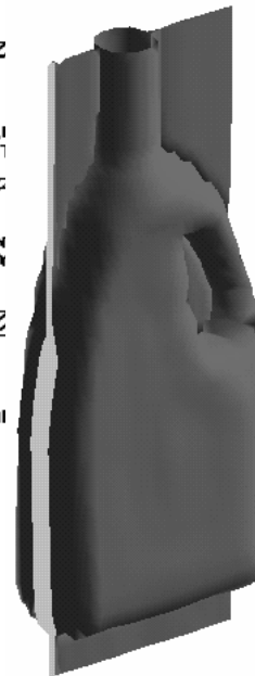
A programmed parison designed to fit a particular mold configuration.
