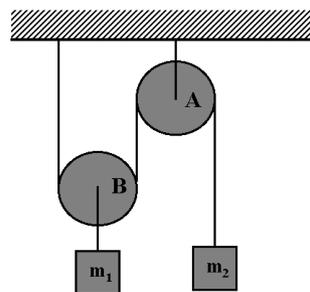
$$\begin{aligned} T_1 - m_1g &= m_1 \frac{a}{2} \\ m_2g - T_2 &= m_2 a. \end{aligned}$$
