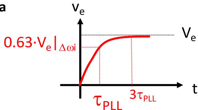
$$v_e(t) = v_{e(t \rightarrow \infty)} + (v_{e(t=0)} - v_{e(t \rightarrow \infty)}) \cdot e^{-\frac{t}{\tau_{PLL}}}$$
