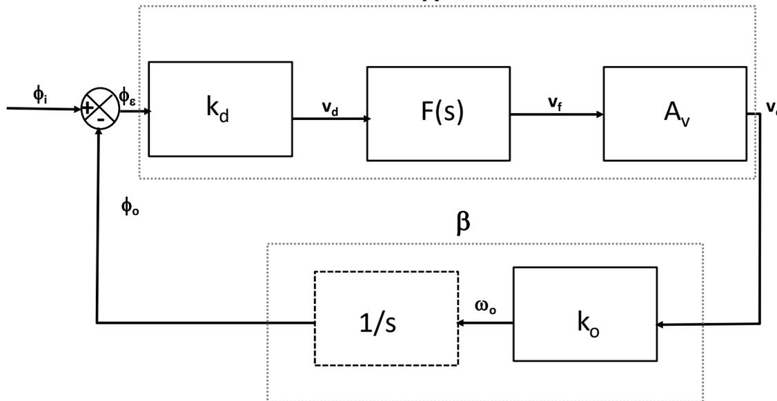
$$\left. \begin{array}{l} \frac{v_e}{\phi_i}(s) = \frac{A}{1 + A \cdot \beta} = \frac{K_d \cdot F(s) \cdot A_v}{1 + K_d \cdot F(s) \cdot A_v \cdot K_o \cdot \frac{1}{s}} \\ \Delta\omega_i = s \cdot \phi_i \end{array} \right\} \Rightarrow \frac{v_e}{\Delta\omega_i}(s) = \frac{K_d \cdot F(s) \cdot A_v}{s + K_d \cdot F(s) \cdot A_v \cdot K_o}$$
