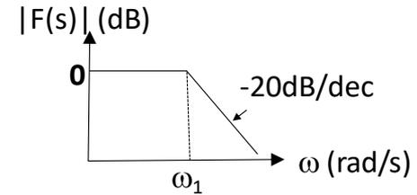
$$\left. \begin{aligned} \frac{v_e}{\Delta\omega_i}(s) &= \frac{K_d \cdot F(s) \cdot A_v}{s + K_d \cdot F(s) \cdot A_v \cdot K_o} \\ \text{Ganancia de lazo } K_V &= K_d \cdot A_v \cdot K_o \end{aligned} \right\} \Rightarrow \frac{v_e}{\Delta\omega_i}(s) = \frac{1}{K_o} \cdot \frac{F(s)}{\frac{s}{K_V} + F(s)}$$
