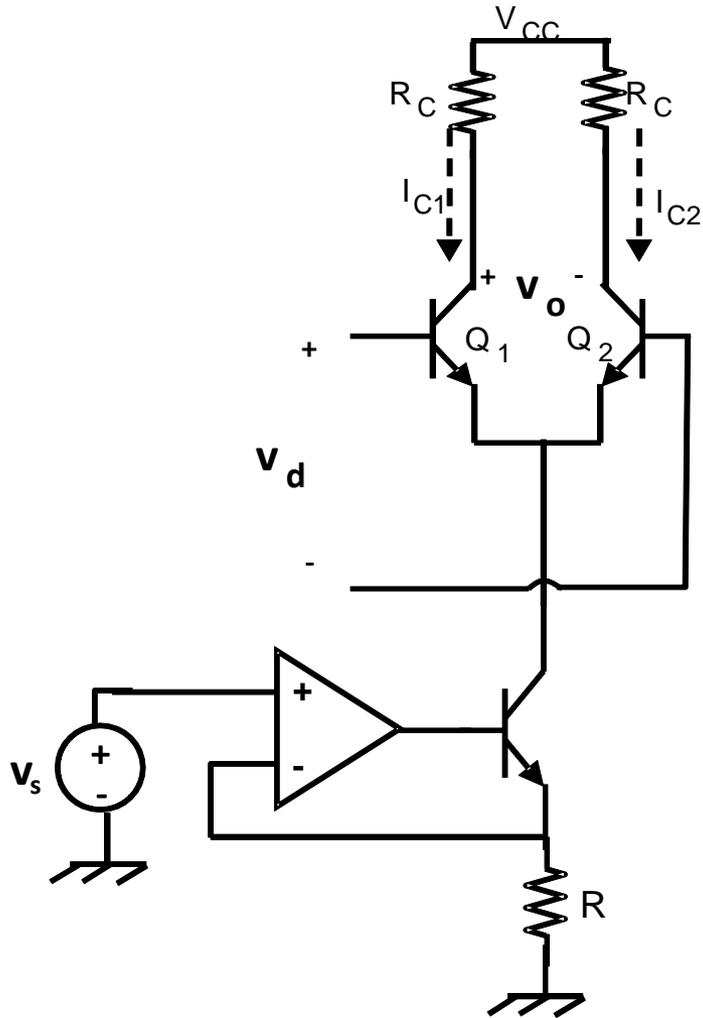
$$V_o = V_{C_{Q1}} - V_{C_{Q2}} = -V_d (g_{m1} - g_{m2}) * R_c$$
