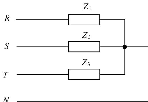
DATOS:  $Z_1 = 6 \angle 0^\circ$        $Z_2 = 6 \angle 30^\circ$        $Z_3 = 5 \angle 45^\circ$
