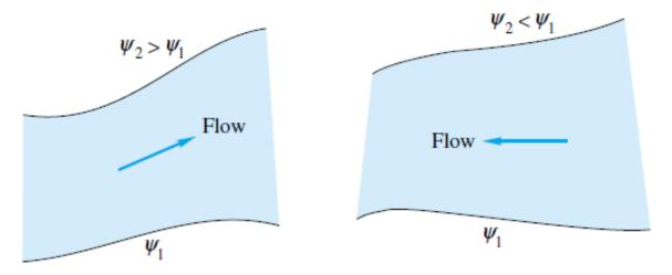
Thus the change in  $\psi$  across the element is numerically equal to the volume flow through the element. The volume flow between any two points in the flow field is equal to the change in stream function between those points:
