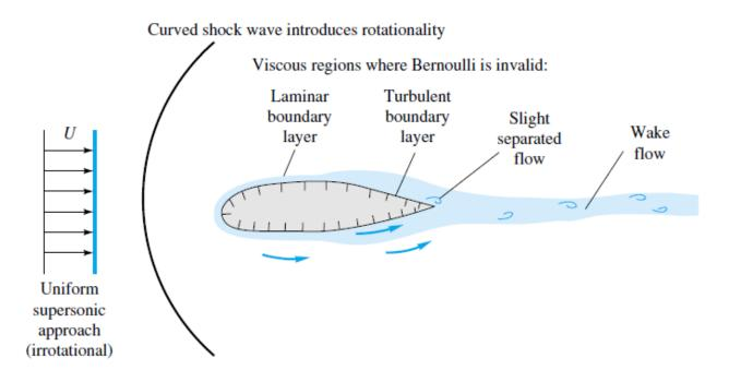
Supersonic flow past a body (U > a); frictionless, rotational flow outside the boundary layer (Bernoulli equation valid, potential flow invalid). the flow downstream is *rotational* due to entropy gradients. Euler's equation can be used in this frictionless region but not potential theory.
