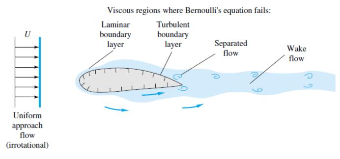
Typical flow patterns illustrating viscous regions patched into nearly frictionless regions: (a) low subsonic flow past a body(U << a); frictionless, irrotational potential flow outside the boundary layer (Bernoulli and Laplace equations valid)
