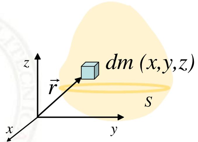
$$x^G = \frac{\int_S x dm}{M}; \quad y^G = \frac{\int_S y dm}{M}; \quad z^G = \frac{\int_S z dm}{M}$$
