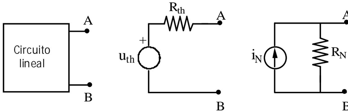
$$R_N = R_{th} \quad i_N = \frac{u_{th}}{R_{th}}$$
