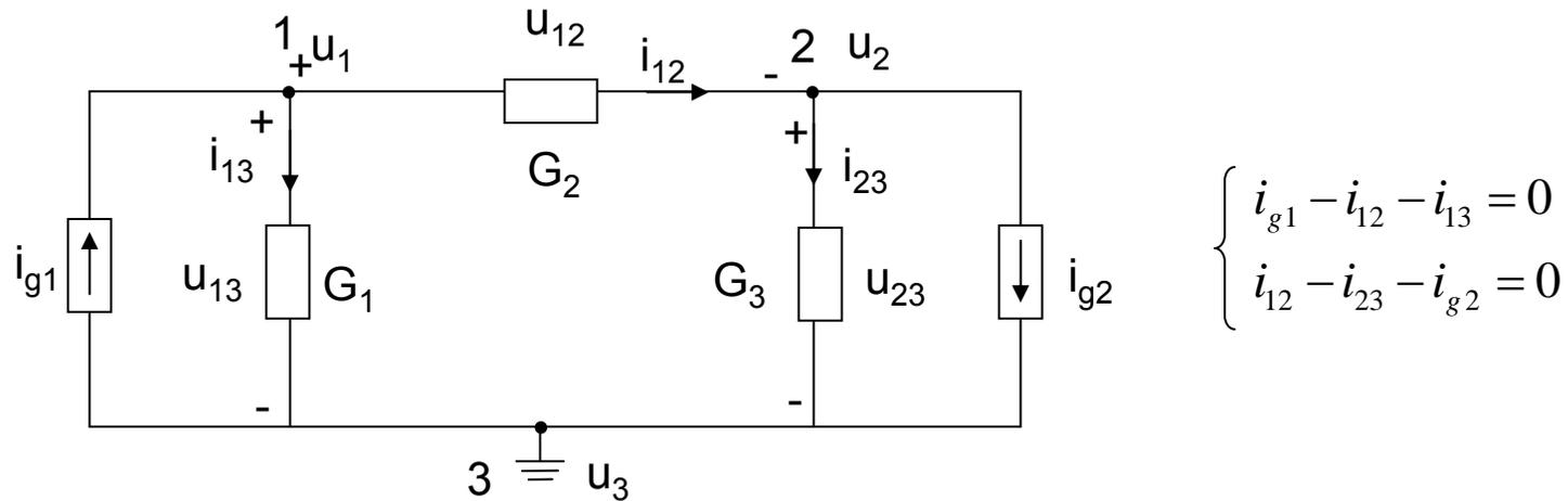
$$i_{12} = u_{12}G_2 = (u_1 - u_2)G_2 \quad i_{13} = u_1G_1 \quad i_{23} = u_2G_3$$
