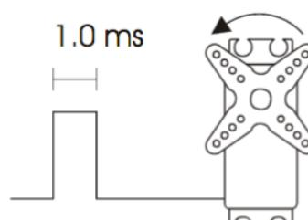
The Pololu servo controller performs the processor-intensive task of simultaneously generating 16 independent servo control signals. The servo controller can generate pulses from 0.25 ms to 2.75 ms, which is greater than the range of most servos, and which allows for a servo operating range of over 180 degrees.
