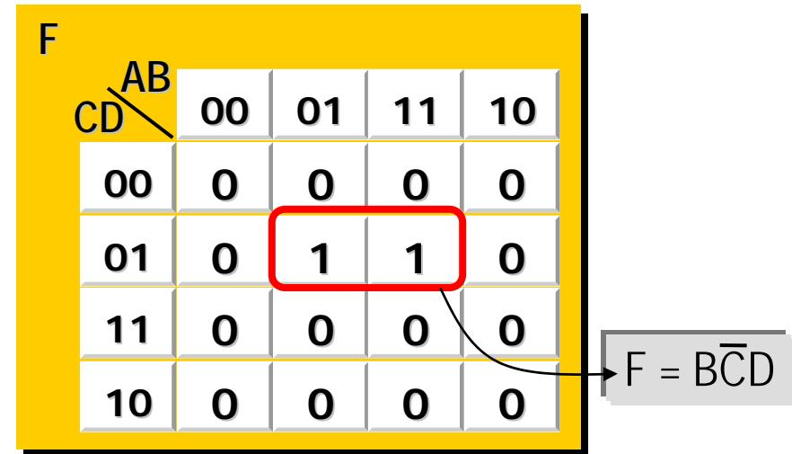
$$\begin{aligned} F &= \overline{A}\overline{B}\overline{C}D + AB\overline{C}D + \overline{A}BCD + ABCD \\ &= B\overline{C}D (\overline{A} + A) + BCD (\overline{A} + A) \\ &= BD (\overline{C} + C) = BD \end{aligned}$$
