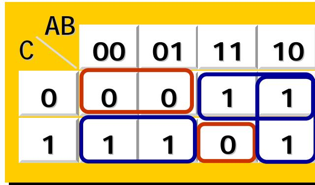
$$D = \bar{A}C + A\bar{C} + A\bar{B}$$
