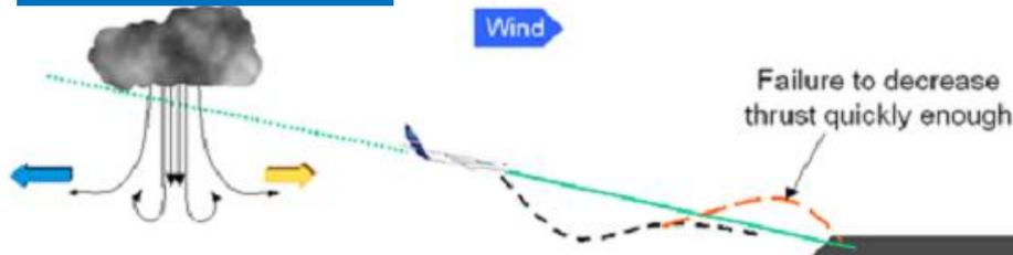
In case of a sudden increase of the tailwind, the aircraft airspeed decreases instantaneously. The lift decreases and the aircraft tends to fly below the intended approach path.
