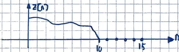
$$\underline{z(k) = \text{DFT}_{16}(z[n]) = \sum_{n=0}^{15} z[n] e^{-j \frac{2\pi}{16} nk} \quad k = 0, \dots, 15}$$
