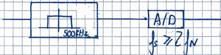
$$f_s \text{ mínima} = 1 \text{ MHz} \quad (2 \times 500 \text{ kHz})$$
