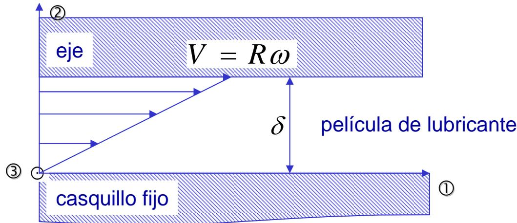
$$\begin{cases} v_1(x_1, x_2, x_3) = R\omega \frac{x_2}{\delta} \\ v_2(x_1, x_2, x_3) = 0 \\ v_3(x_1, x_2, x_3) = 0 \end{cases}$$
