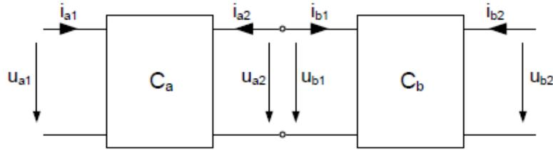
$$\begin{pmatrix} u_{a1} \\ i_{a1} \end{pmatrix} = [A_a] \cdot \begin{pmatrix} u_{a2} \\ -i_{a2} \end{pmatrix} \quad y \quad \begin{pmatrix} u_{b1} \\ i_{b1} \end{pmatrix} = [A_b] \cdot \begin{pmatrix} u_{b2} \\ -i_{b2} \end{pmatrix}$$
