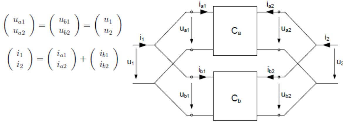
$$\begin{pmatrix} u_{a1} \\ u_{a2} \end{pmatrix} = \begin{pmatrix} u_{b1} \\ u_{b2} \end{pmatrix} = \begin{pmatrix} u_1 \\ u_2 \end{pmatrix}$$
