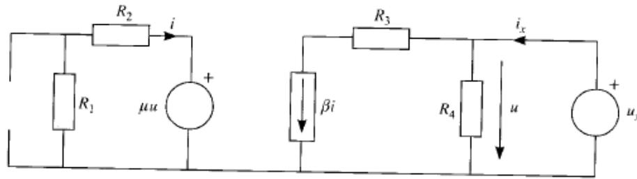
$$i_x = \frac{u_x}{R_4} + \beta i \quad i = -\frac{\mu u_x}{R_1 + R_2}$$
