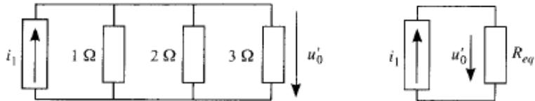
$$u'_0 = R_{eq} \cdot i_1 = \frac{1}{\frac{1}{1} + \frac{1}{2} + \frac{1}{3}} i_1 = \frac{6}{6 + 3 + 2} i_1 = \frac{6}{11} i_1$$
