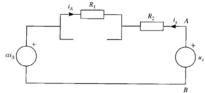
$$u_x = R_2 i_x + R_1 i_x - \alpha i_x = (R_2 + R_1 - \alpha) i_x$$
